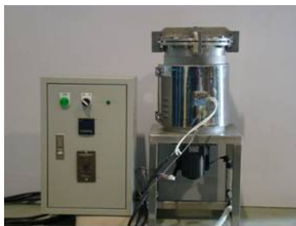
Fig. 1. Teflon-lined stainless steel autoclave unit.
